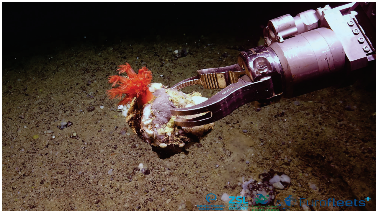
Figure 1: Collection of sample using the ROV manipulator.
